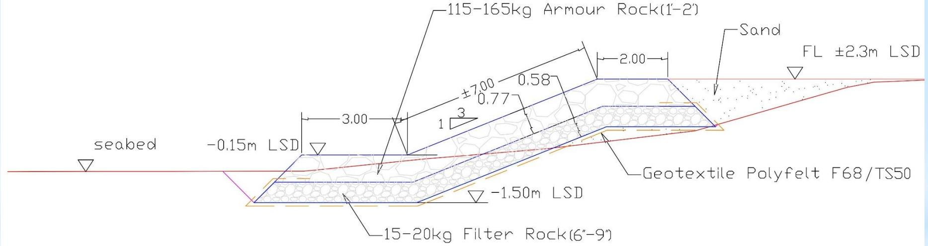
TYPICAL SECTION OF ROCK REVETMENT WORK
